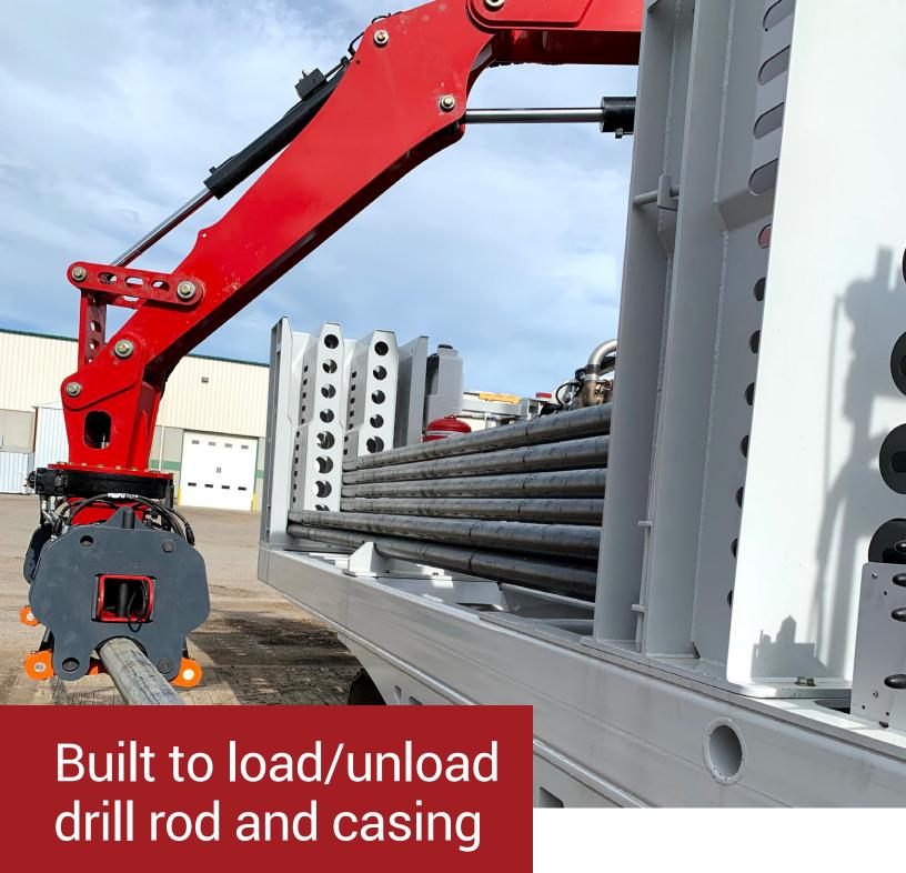
Introducing hydraulic robotic rod handling. The Borterra RodBot™ can be adapted for virtually any piece of drilling equipment.
