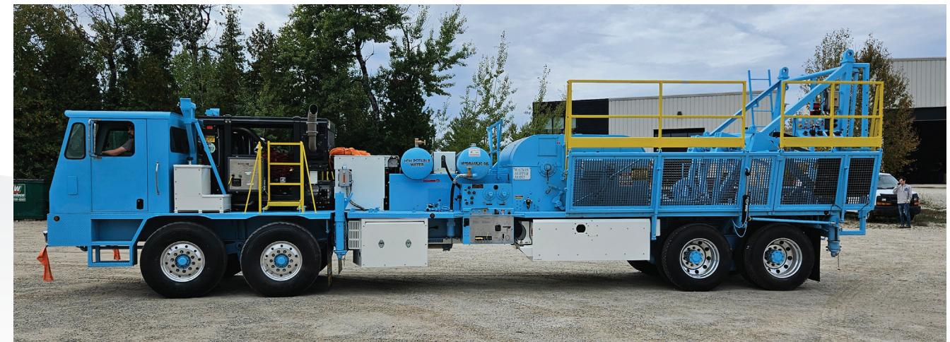
Once Colorado-based Watson Hopper partnered with MEDATech, it was able to offer a hybrid diesel/battery-electric retrofit that outperforms diesel workover rigs while cutting noise, fuel use, and emissions.
