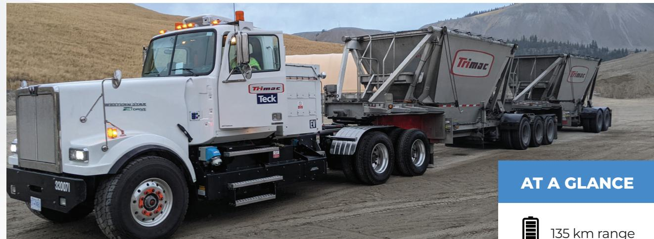
In a mining industry first, MEDATech converted a Western Star 4900XD into a battery-electric haul truck for Teck Resources. Since 2022, it has transported concentrate from Highland Valley Copper mine to a rail terminal in B.C. powered by the MEDATech AltDrive system.
